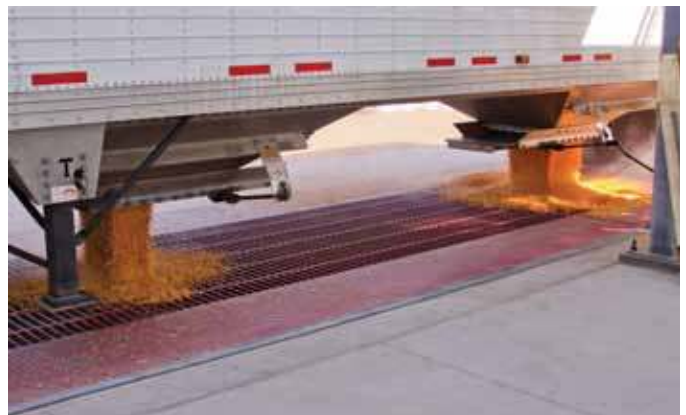
The scale's custom section allows grain to flow through to underground conveying equipment.
